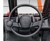
Small-diameter Steering Wheel The small-diameter steering wheel with the full hydraulic power steering system provides excellent maneuverability.
