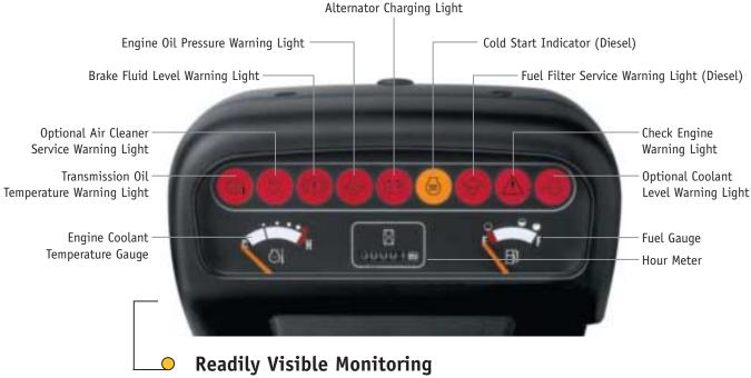
The instrument panel tilts with the steering wheel for sustained visibility and provides easy monitoring of truck functions plus early warnings of potential problems to promote preventive maintenance.
