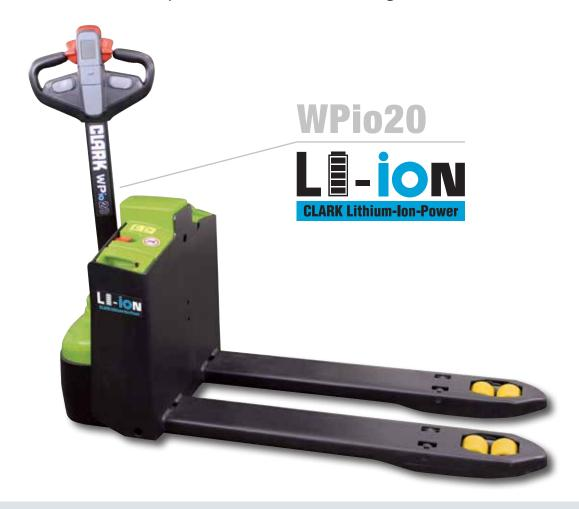
For Medium and more Intensive Applications Integrated Charger, Castor Wheels, Smart Display, Storage Compartment Small Lamp in the Lithium-ion Battery Provides Light In Dark Storage Areas
