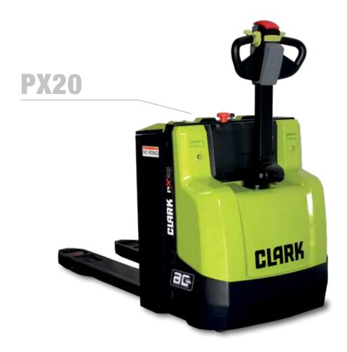
For Intensive Applications Solid forks, Robust Metal Frame and Powerful AC-Drive Motor Battery Capacity from 150 Ah to 375 Ah
