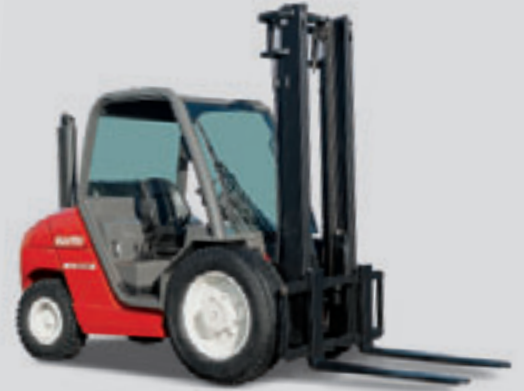
MSI 30 G with fixed reservoir (standard version with gas bottle).
