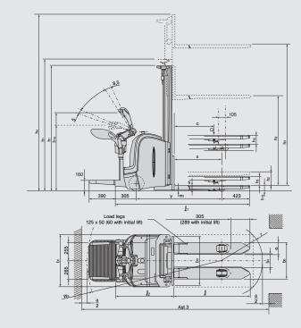
Aisle width Ast = Wa + r + a (Safety clearance a = 200 mm)
