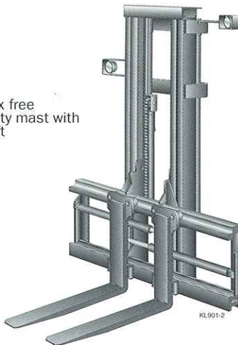
Triplex free visibility mast with free-lift 90-136, two free-lift cylinders (150-180, one central free-lift cylinder)
