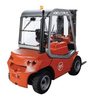
**C4D400E-500E** (4.5 litre diesel engine) Sheer power and strength for heavy-duty handling, with capacities of 4000, 4500, and 5000kg. Exceptional power at low revs—58kW at just 2000rpm.
