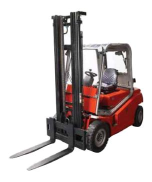
C4D150D-200D (2.5 litre diesel engine) **C4G150D-200D** (2.2 litre LPG engine) These compact models offer capacities of 1500, 1800, or 2000kg, and offer maximum power at low revs giving effortless performance.
