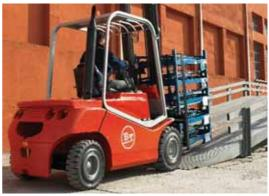
Starting the truck is a two-stage process: key and start button. For extra safety, it is also necessary for the hand operated parking brake to be applied before the truck can be activated. The emergency cut-off button kills hydrostatic pressure, thereby immediately disabling the truck.
