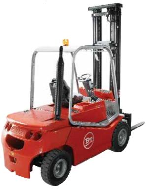
**C4D250E-350E** (3.3 litre diesel engine) **C4G250E-350E** (2.2 litre LPG engine)
