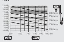
Lifting capacity diagrams valid with SE-tyres.
